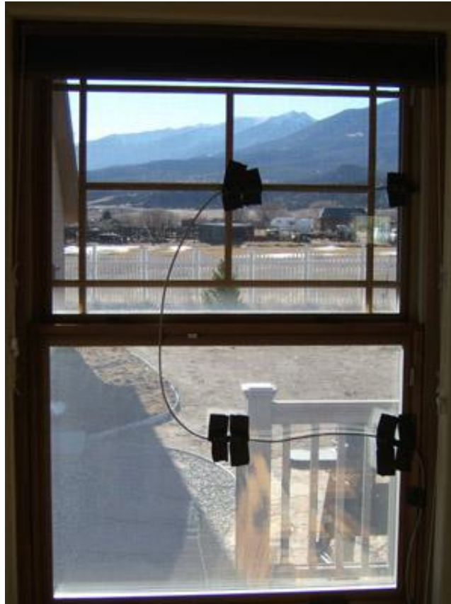
Figure 6. Location of the Four T-Sense™ Temperature Sensors on each Window.
